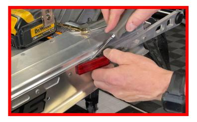
Using the T30 Torque bit and 10mm end wrench, remove the two bolts on each side of the bumper which holds the bumper to the tunnel. Once both sides are removed, the Bumper will be free and easily removed.
