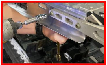
Take the new ZBROZ Rail Plates and line them up against the factory rail to ensure the rivet wholes and handle bolts line up.
