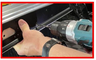
Now make sure you have drilled out the last 4 four holes at the end of the tunnel. Take the ZBROZ Grab Bar Plate and place it on the end of the tunnel overtop of the ZBROZ plate. The 4 holes should line up.
