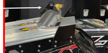
Take the Billet Cross Bar and place it on the inside of the cross bar plates lining up the wholes with the cross bar threaded whole.
